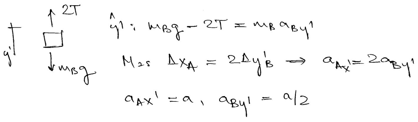
$$\begin{aligned} T - \mu m_A g &= m_A a && \times 2 \\ m_B g - 2T &= m_B a/2 && \downarrow \oplus \end{aligned}$$
